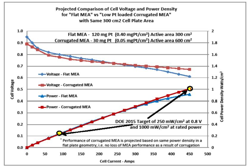
Take-Away: If low Pt loaded MEA is built in the "Corrugated MEA" configuration, it achieves the DOE Power Density targets of 250 mW/cm<sup>2</sup> and 1000 mW/cm<sup>2</sup> at low and rated power. (Read Project Goal)
