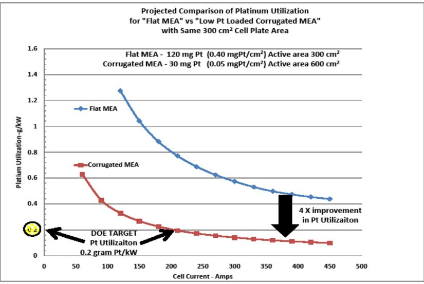
Take-Away: And Corrugated geometry allows to meet DOE Target Pt utilization of 0.2 g Pt/kW (Read Project Goal)
