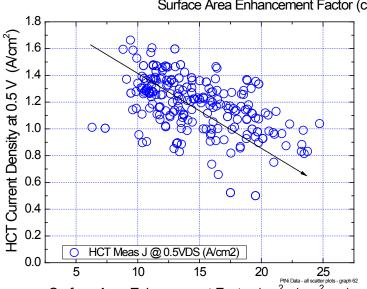
Excess Ni at higher loadings further reduces limiting currents.
