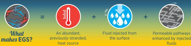
With an enhanced geothermal reservoir, you can generate power anywhere with hot rocks at depth!
