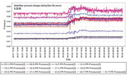
Figure 5: Under-floor pressure improvement from floor-tile tuning. Courtesy: SynapSense Corp.
