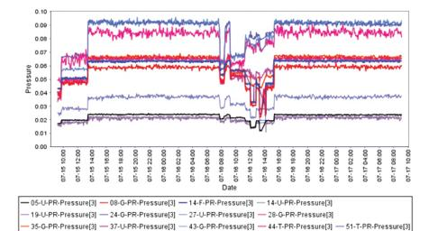
Figure 7: Verify the impact of CRAC maintenance by observing under-floor pressure. Courtesy: SynapSense Corp.
