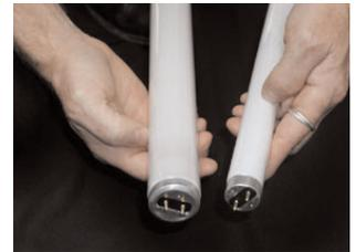
T12 lamps are an older technology and should be replaced with T8 lamps in your facility. T8 lamps provide superior lighting quality and last longer, while improving efficiency by 30%. They also operate on electronic ballasts that are more efficient than older magnetic ballasts, which are common among fixtures using T12 lamps.
