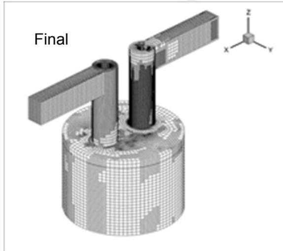
Initial and final grids at given crank angle
