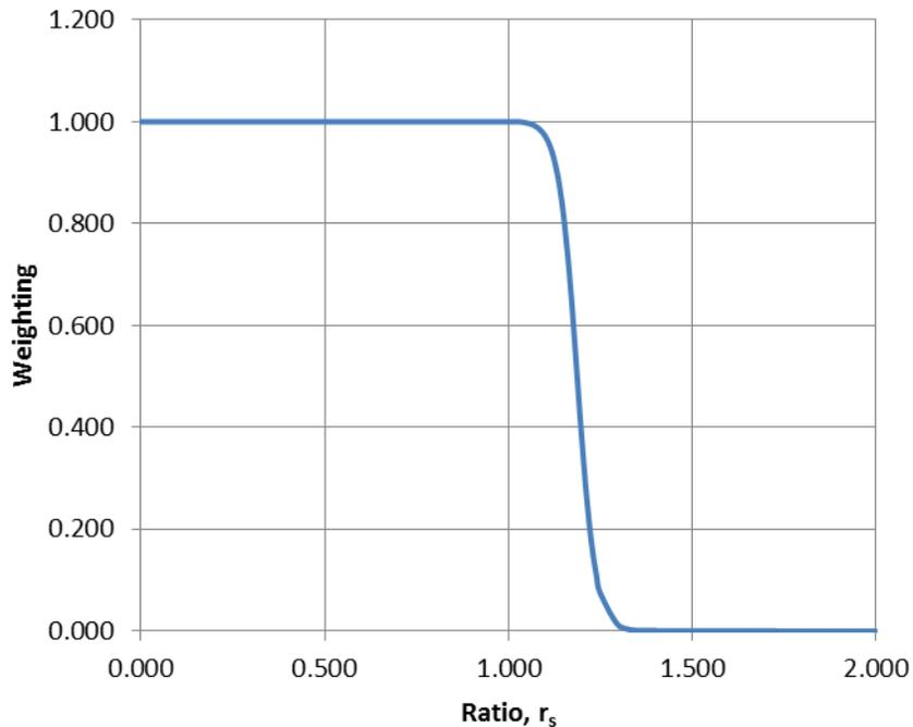
**Figure B-2. Score weighting based on rpm ratio for control of rated rotor speed task**
