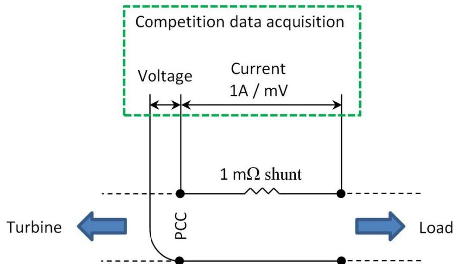
**Figure 2. Load, turbine, and point of common coupling arrangement**
