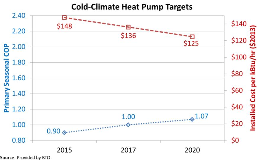
**Figure 1-10: Cost and efficiency targets for cold-climate heat pumps**
