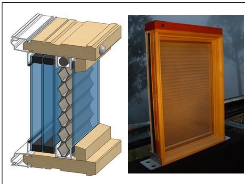
Figure 19. Highly insulating, dynamic windows with automated shading, schematic diagram (left) and prototype (right) (images courtesy of LBNL)
