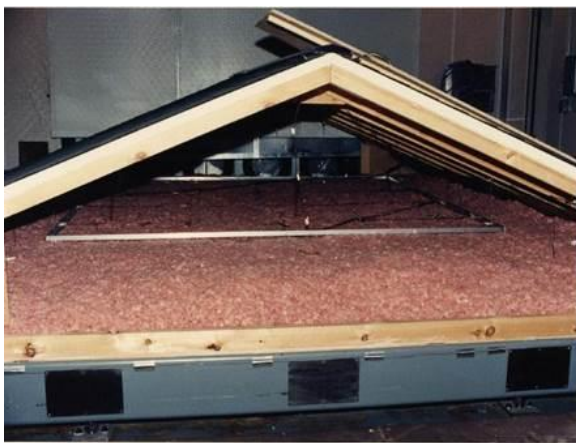
Figure 26. Fibrous glass loose fill insulation installed in a test attic in a climate simulator just prior to evaluating its R-value.
