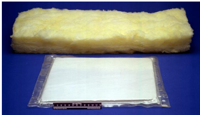
Figure 23. The VIP in the foreground has an R-value three times higher than the fibrous batt insulation in the background at one-third the thickness.
