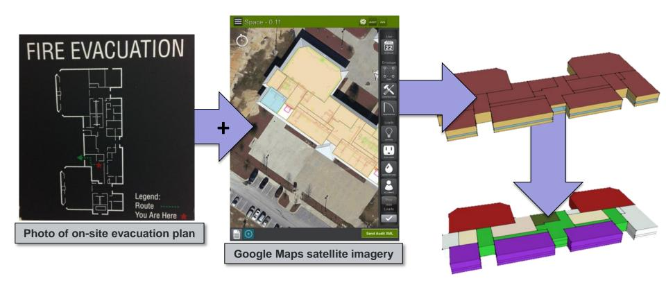
OpenStudio automatically generates a detailed energy model ready for simulation
