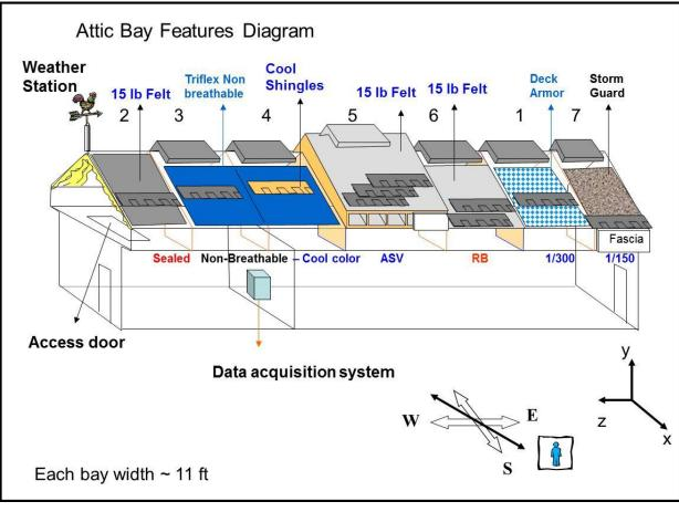
Breathability: < 0.1 perm vapor impermeable > 1.0 and < 10.0 perm semi permeable
