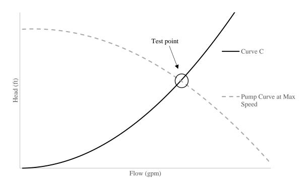
Figure III.2. Specified Load Point on Curve C at Maximum Speed for Single-Speed Self-Priming and Non-Self-Priming Pool Filter Pumps.
