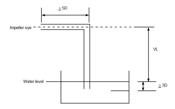
**Figure III.6. Test Apparatus for Testing of Self-Priming Capability for Pool Filter Pumps.** (In the Figure, D = nominal riser pipe diameter and VL = vertical lift, which much be at least 5.0 feet, adjusted to a nominal conditions. Source: NSF/ANSI 50-2015, figure C.1.)
