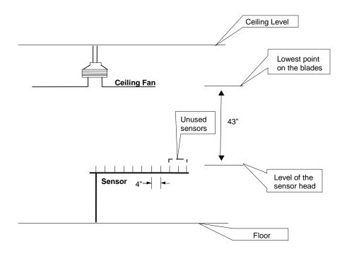
Figure 2 to Appendix U to Subpart B of Part 430: Air Delivery Room Set-Up for Ceiling
