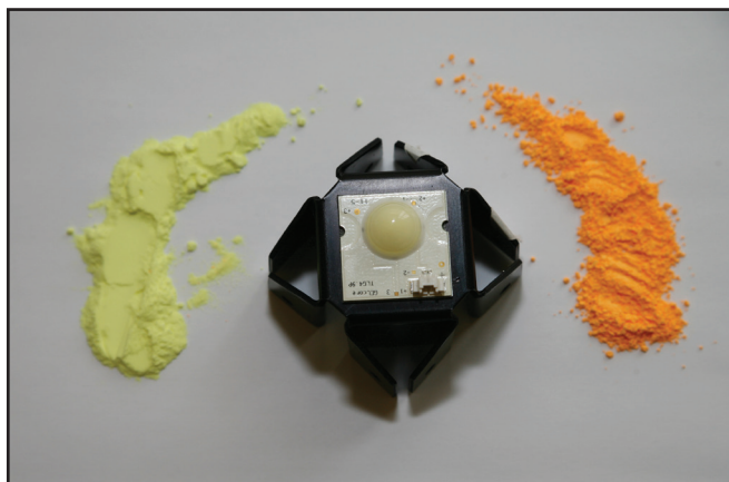
GE's Optimized Phosphors and LED Light Engine
