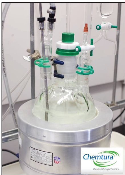
Chemtura's Synthetic Refrigerant Lubricant Lab-Scale Manufacturing Process
