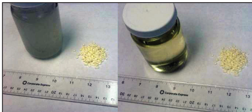
Syntroleum's PCM (wax/solid form T < 22^\circ\text{C} [L] and molten form T > 23^\circ\text{C} [R])
