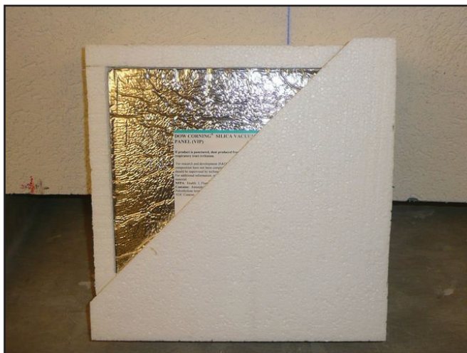
VIP Encapsulated in EPS for Use in a High-Performance EIFS Wall
