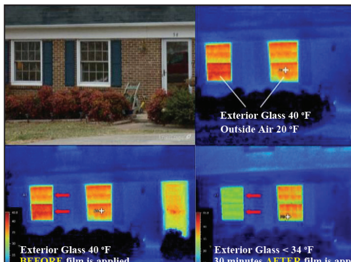
Solutia's Low E-Film Technology Before and After Installation
