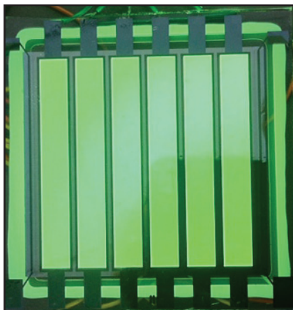
PPG's Substrate Used in a Green Phosphorescent OLED "Vertical Blind" Made by UDC
