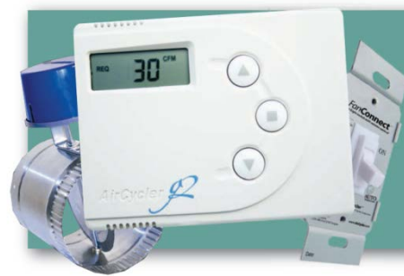
Installed inside AHU, totals OA flow hourly. Closes electronic damper in OA duct or runs bathroom to match hourly flow to 62.2 target
