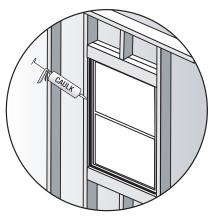
• On the interior side of the window, seal the gap between the window and the rough opening with a backer rod or non-expanding foam and caulk.
