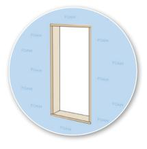
**STEP 3** Install the exterior foam. The outer face of the foam should be flush with the outer edge of the plywood frame.
