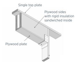
Closed, insulated headers are one advanced framing technique. (*Figure source: CARB*)
