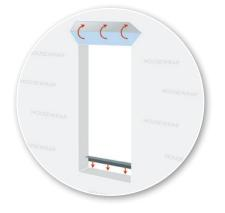
**STEP 5** Fold in housewrap at jambs and sill. Fold back temporarily at jamb. Install backdam on sill.
