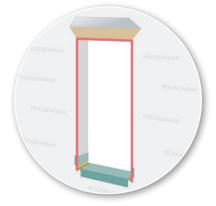
**STEP 5** Apply sealant at jambs, head, and sill.
