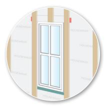
**STEP 10** Install vertical wood strapping on top of the foam and housewrap to use when attaching siding.
