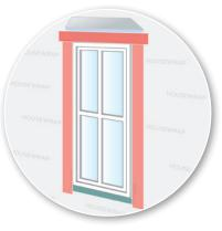
**STEP 8** Install jamb flashing first; install a drip cap (if applicable); install head flashing.
