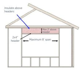
Using single 2x4 headers instead of double 2x6 headers in non-load-bearing walls allows space for insulation.
