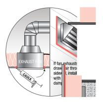
Provide bathroom and kitchen exhaust fans. Duct them to the outside and caulk ducts at the dry wall for an air-tight seal. Use low-sone fans for quiet operation.
