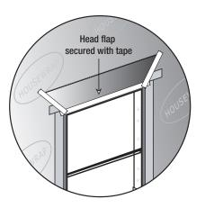
If a head flap was created, fold it over the head flashing and tape across the top window flange and the 45° angle seams.
