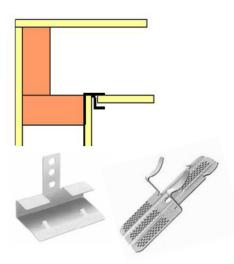
Two-stud corners with drywall clips use the least wood and give the best thermal performance.
