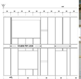
*(left)* Sheet goods come in 4x8-foot dimensions. Designing and building on a 2-foot grid saves cutting time and reduces lumber and sheet good waste.
