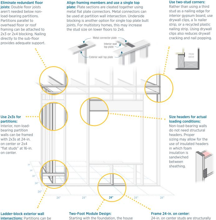
**intersections:** Partitions can be nailed either directly to a single exterior wall stud or to flat blocks inserted between studs. Starting with the foundation, the house footprint should be based on 2-foot increments. Layouts should be based on this 2-foot grid to minimize material waste.
