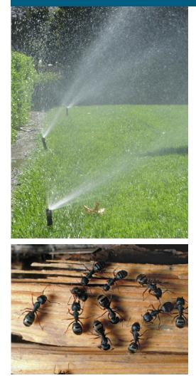
*(top)* Place plants at least 18 inches from finished structure and direct irrigation away from the foundation.
