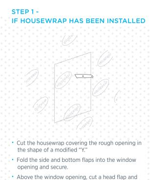
Above the window opening, cut a head flap and flip it up to expose sheathing, and loosely tape in place out of the way.
