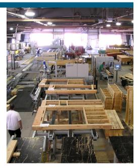
Quadrant Homes, a Building America builder in Bellevue, Washington, builds its wall panels in a factory to ensure consistency and shorten site construction time.
