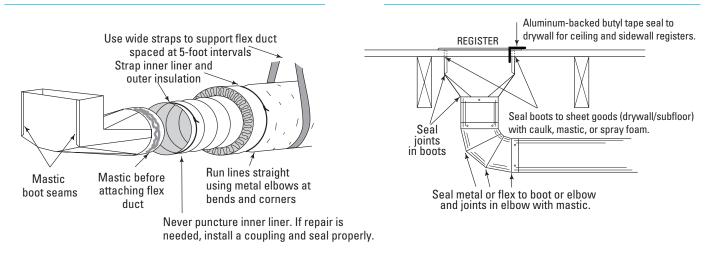
Mastic is a gooey adhesive that is applied wet. It fills gaps and dries to a soft solid. Mastics may or may not contain reinforcing fibers, and they may be used with reinforcing mesh tape.
