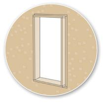
**STEP 2** Line rough opening with a frame made of plywood strips <sup>3</sup>/<sub>4</sub>" thick by wall dimension + width of foam (the plywood should be flush on the interior surface and extend to the anticipated outside face of the foam).
