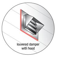
Dryer vent exhausts must have a closeable gravity or automatic damper. A single hinged door with a  $2\frac{1}{2}$ -inch effective opening is not as effective as a louvered damper.
