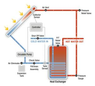
This solar water heater uses propylene glycol (antifreeze) in the exposed collector, making it safe for use when temperatures are below freezing. The glycol loop heats up on the roof then passes through the tank of potable water to release its heat then it is pumped back to the roof to reheat.
