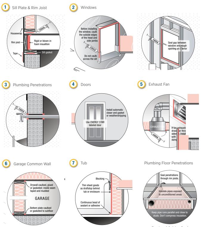
Keep pipes out of exterior walls and seal penetrations through floor.
