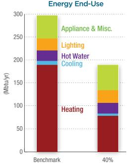
A Comparison of Energy Usage by End Use for a Home Built to Perform with 40% Energy Savings Compared to the Building America Benchmark (a home built to MEC 1993) in the Cold Climate. *Example based on a 2-story, 1,354 ft<sup>2</sup> house in Pasco, WA. Analysis by BIRA.*
