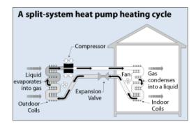
In heating mode, an air-source heat pump evaporates a refrigerant in the outdoor coil. As the liquid evaporates, it pulls heat from the outside air. After the gas is compressed, it passes into the indoor coil and condenses, releasing heat to the inside of the house. The pressure changes caused by the compressor and the expansion valve allow the gas to evaporate at a low temperature outside and condense at a higher temperature indoors. In cooling mode, the reverse happens.
