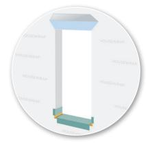
**STEP 6** Install adhesive-backed sill flashing and corner flashing patches at sill. Apply sealant at jambs, head, and sill.
