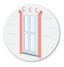
**STEP 9** Fold down head housewrap; apply corner patches at head; air seal window around the entire perimeter on the interior with sealant or non-expanding foam.
