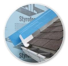
**STEP 5** Apply self adhesive flashing over top of wall flashing, diverter and rigid foam insulation.
