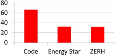
ES and ZERH used similar heating energy because the mini-split heat pump unexpectedly operated at about the same COP as a traditional, split system heat pump.
