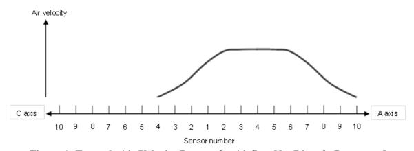
Figure 1: Example Air Velocity Pattern for Airflow Not Directly Downward
