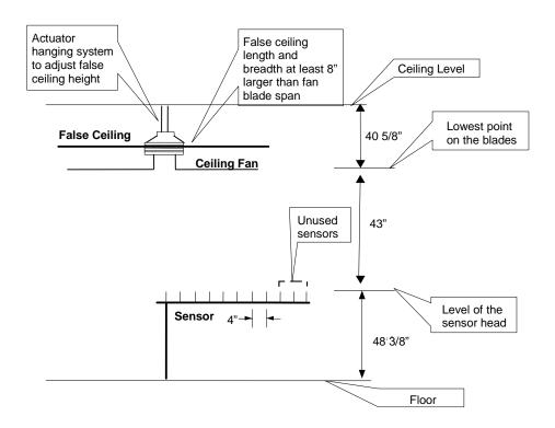
Figure 2: Air Delivery Room Set-Up For Low-Volume Ceiling Fans
