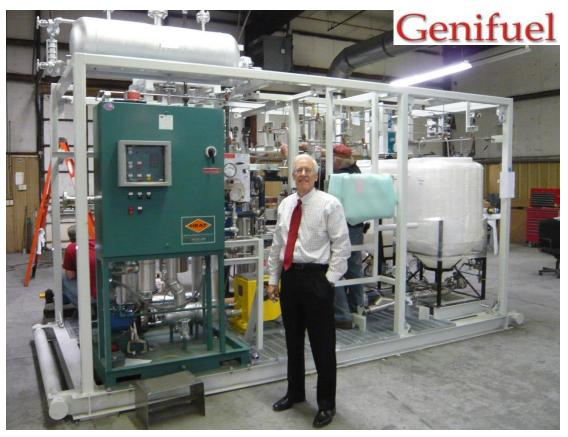
Jim Oyler with the 1000 L/day (of 20 wt% BDAF) Hydrothermal Processing Pilot System continuous HTL/CHG system for algal feedstock NAABB-Reliance-PNNL-Genifuel
