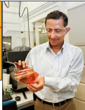
Low-cost wireless sensor prototype on flexible substrate
