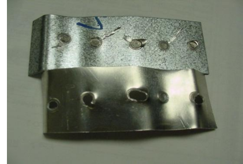
Direct resistance spot welds made between 1-mm Al and 0.8-mm galvanized steel sheet
