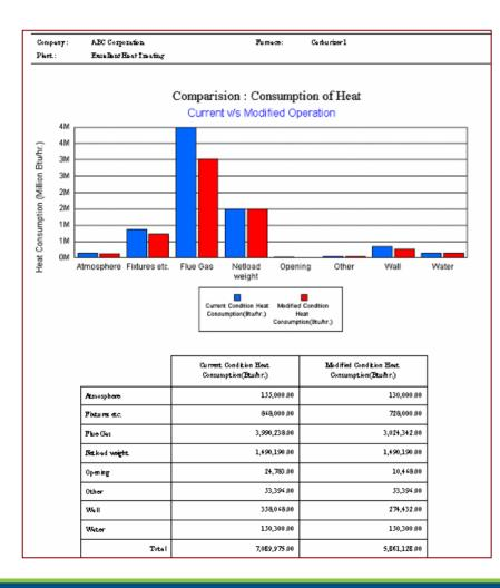
Compares energy use for current operations and with potential changes (what-if analysis) in operating conditions for the furnace.
