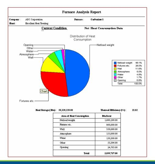
Analysis of energy used in part of a furnace under a given operating condition.
