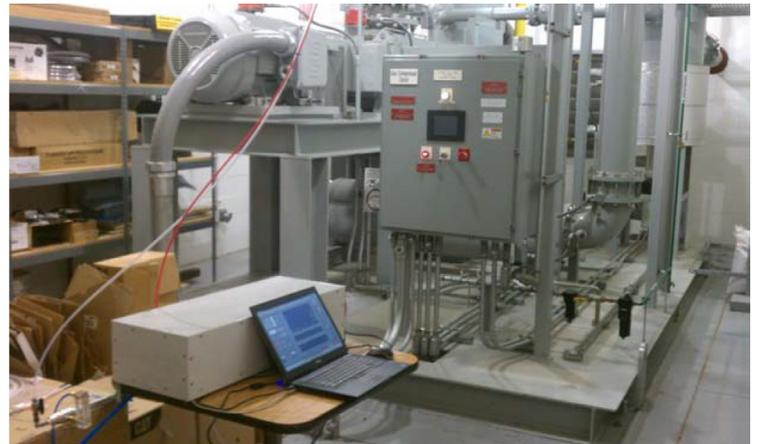
A gas quality sensor (GQS) setup at Bath Landfill, Steuben County, NY. Real-time GQS technology and engine control system improvements are addressing fuel quality issues with opportunity fuels such as landfill gas and digester gas.
