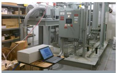
A gas quality sensor (GQS) setup at Bath Landfill, Steuben County, NY. Real-time GQS technology and engine control system improvements are addressing fuel quality issues with opportunity fuels such as landfill gas and digester gas.
