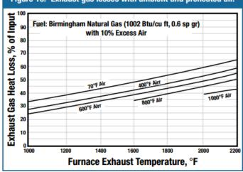
Figure 10. Exhaust gas losses with ambient and preheated air.
