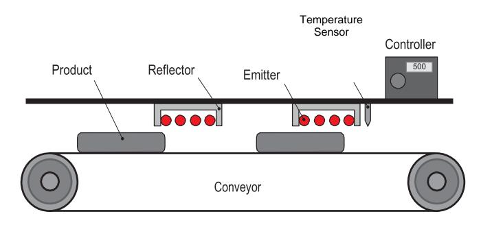
Figure 4. Simple schematic of an electric infrared heating system
