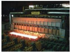
A walking beam furnace for metal reheating
