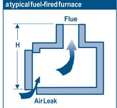
Figure 1. Air leakage and gas flow in
