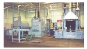
A quench furnace line for heat treating
