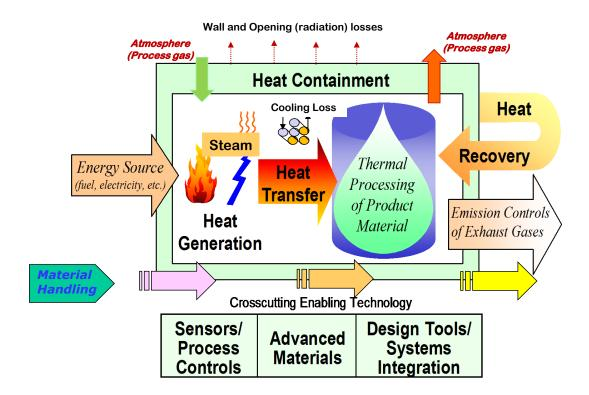
Figure 1. A fuel-based process heating system and opportunities for improvement Fuel-based process heating equipment can be classified in many different ways, including:
