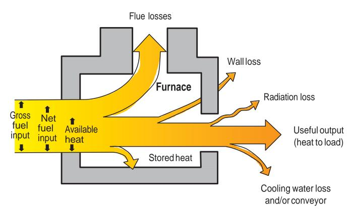
Figure 2. Energy loss diagram in a fuel-based process heating system.
