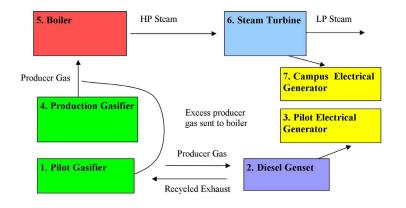
Energy-flow schematic for use of a producer gas-powered genset. Illustration courtesy of University of Minnesota Morris
